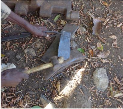
**FIGURE 17** Demonstration of usage of blacksmithing tools: a metal rod held over an anvil with a tong and struck with a hammer, Aṭeyä (B. Kribus/V. Krebs)
