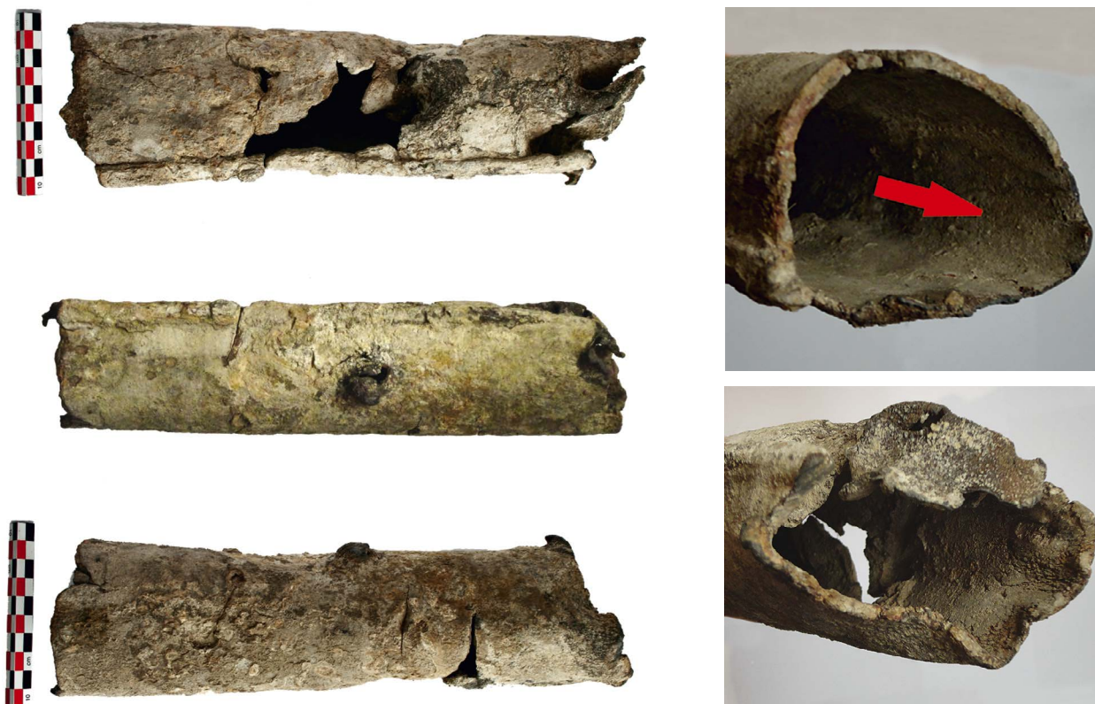
Figure 7. Lead pipe fragment from Horia, near Troesmis (sampled as RO-2). Total recording (left), close-up with red arrow marking the sampling spot and close-up from the hardly damaged end (right). Photos: (left) C. Bodea (ICEM), (right) C.-G. Alexandrescu.
