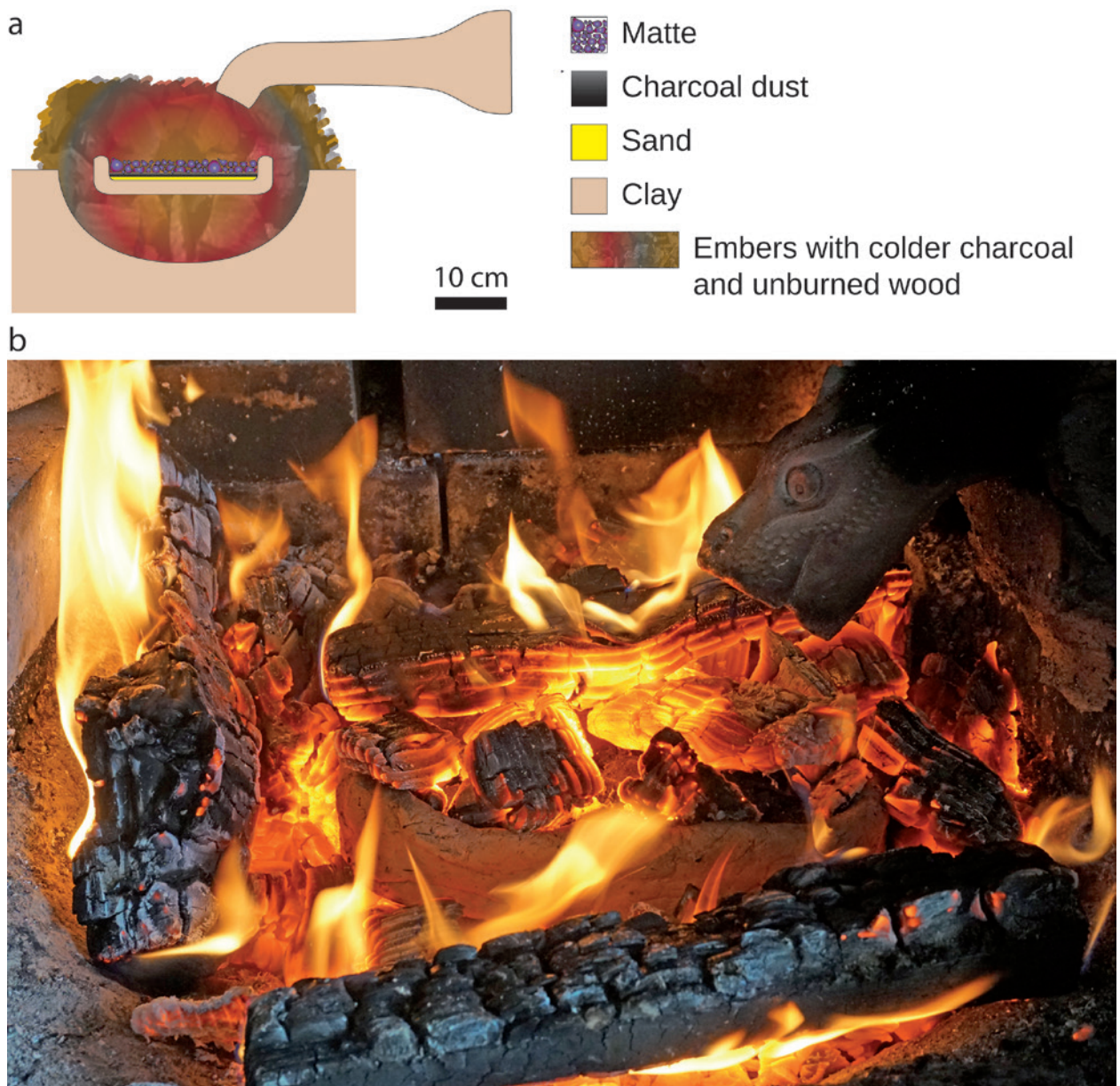
Figure 6. Smelting of the enriched matte, a) sketch of the experimental set-up; b) photograph of the fire pit (modified after Rose, Hanning and Klein, 2019).
