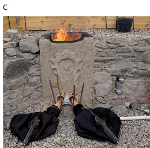
Figure 3. Smelting of the roasted ore, a) sketch of furnace; b) temperature curve; c) front view of the furnace with bellows and tuyères; d) furnace conglomerate (modified after Rose, Hanning and Klein, 2019).
