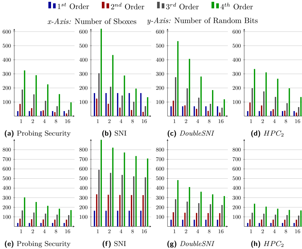
Figure 8: Randomness requirements per S-box (in average) when implementing multiple AES S-box instances in parallel. The first row shows the results corresponding to the strict clustering while the second row to the relaxed clustering. The data corresponding to 1 st order is drawn from the standard randomness assignment and shown for comparison.
